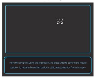
3 After configuring settings is completed, press the Enter key of the JOG button. The aim point is fixed to the specified position and the settings screen disappears.
