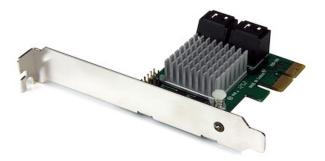
The PEXSAT34RH 4-Port PCI Express 2.0 SATA Controller Card with HyperDuo adds 4 AHCI SATA III ports to a computer through a PCIe slot (x2), delivering multiple internal 6Gbps connections for high-performance hard drives and Solid State Drives (SSDs).
