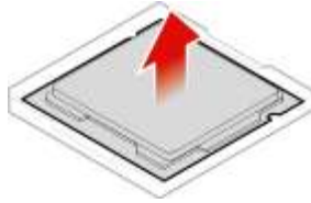
Figure 113. Pivoting the microprocessor socket upward
