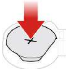
Figure 123. Pressing the coin-cell battery downward until it is fully engaged with a click
