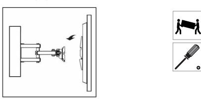
3. Tighten the screws in both mounting arms to secure the display onto the wall, as shown in the figure below.
