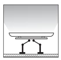
2. Attach the bubble level right at the center of the horizontal TV plate. If the bubble is centered between the lines, it means that mount is correctly positioned on the surface.
