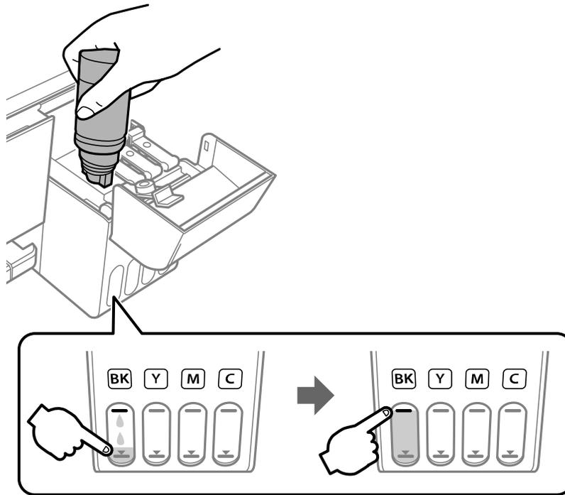
**Note:** If ink does not flow from the bottle, lift and reinsert the bottle.
